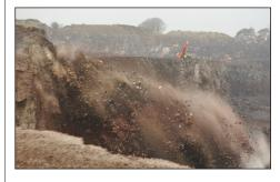
The overall result of each blast is dependant upon all of these factors being appropriately considered, along with the loading density and strength of explosives used, the detonator initiation timing and stemming (sealing them) of the holes prior to initiation.
